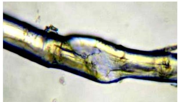
**Figure 3.** Microscope image of a single linen fiber colored with ArF laser. The mechanical damage in the middle shows a colorless inner medulla. Contrast-enhanced detail of figure 8 in Ref. [24].
