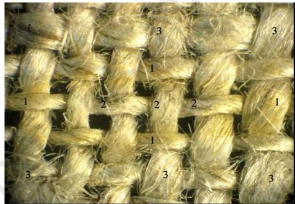
**Figure 2.** The linen area irradiated by ArF laser pulses shows different characteristics corresponding to the local laser intensity value  $I(x,y)$ . 1) colored area; 2) ablated area; 3) area irradiated below threshold for coloration. From Ref. [24].
