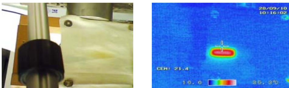
**Figure 13a.** Left: photo of the linen during XeCl laser irradiation. On the right, the same picture seen in infrared light. The color scale at the bottom shows that the warmest region of the linen (in the middle of the laser spot) reaches 33  $^\circ\text{C}$ , while the non-irradiated area is at the room temperature of 20  $^\circ\text{C}$ .
