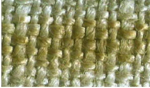
**Figure 3.** Micro-photographs of the cloth irradiated with 100 XeCl laser pulses. Intensity (fluence) on linen  $16 \text{ MW/cm}^2$  ( $0.5 \text{ J/cm}^2$ ) per pulse.
