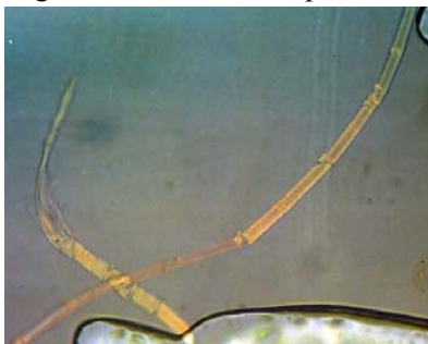
Figure 3. Two sharply terminated image fibers. The individual image fibers have very sharp boundaries at their ends across the 15-micron diameter of the fibers. At the boundary between the image fiber and the clear fiber, there is a sharp change. The imaged areas of the fibers are brittle and are cracked because Frei used his fingernail to crease the sticky tape sharply on the cloth (1978 Frei sample slide 4bd).
